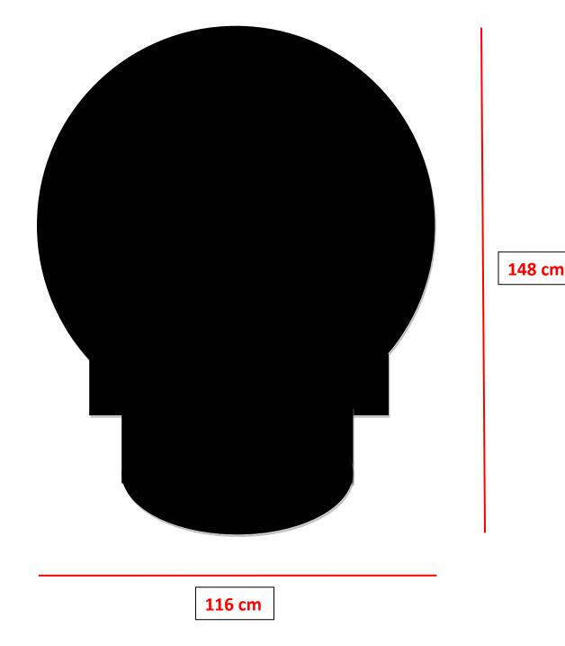
Dimensions are approximate. Amount of mortar used in shell joins and thickness of external plaster will vary. The Alfresco Pizza Oven will fit neatly on a 120cm wide x 130cm deep concrete bench top with the mantle sticking 18cm past the bench top edge. The bench top should be steel reinforced and minimum 8cm thick. 10cm will provide better thermal performance.
